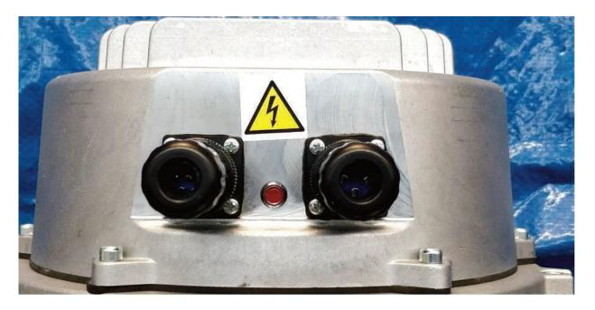
INSERT THE POWER AND SIGNAL CONNECTORS INTO THE MANAGEMENT CARD, TAKING CARE TO MATCH THE PIN (1), WITH THE SLOT (2).
