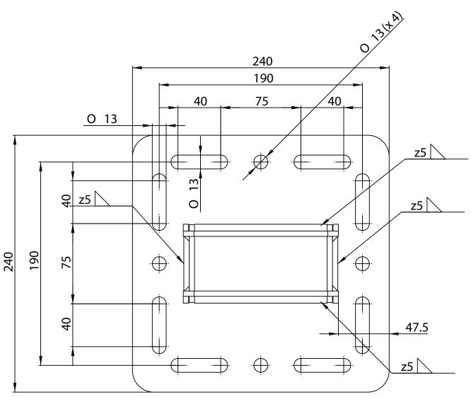
PLACE ROD INTO ROD HOLDER AND FIX WITH SCREW, NUTS AND BOLTS ASSEMBLY POSITION FOR ROD HOLDER DEPENDS ON INSTALLATION STUDY AND DESIGN
