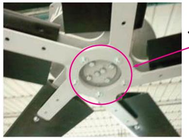
Fix without tightening the 5 central
