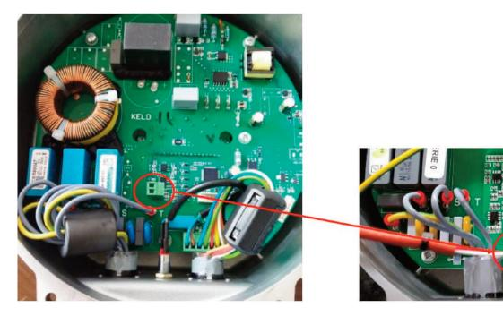
NSERT THE GREEN CONNECTOR, WITH THE WHITE/RED WIRES, OF THE ENGINE TEMPERATURE SEN-SOR INTO THE SPECIAL CONNECTOR ON THE ELECTRONICS (AS POSITIONED IN THE FIGURE).
