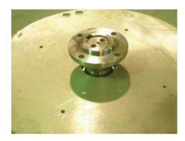
AFTER DISASSEMBLED BLADE SUPPORT, DISASSEM-BLY HUB
